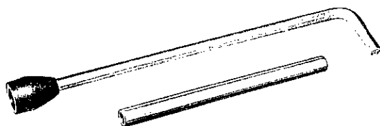
Angled driver for hexagon socket with holder and extension.
